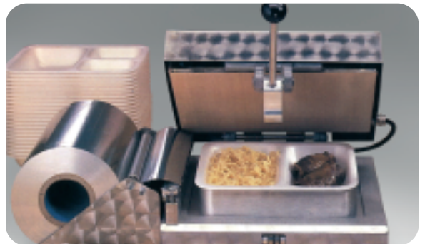
PTFE coated glass fabric at custom width on a Heat Sealing Machine
